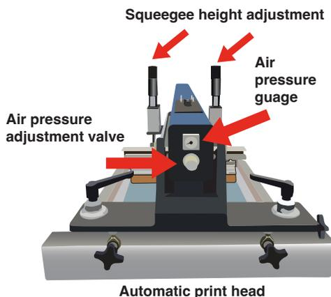
Some presses will only have a squeegee height adjustment to allow you to add more downward pressure to the squeegee. It is important to understand that this adjustment is only for controlling how far downward the squeegee will move. This adjustment will add downward force, but if your print head is equipped with an air pressure regulator, like in the image above, you should use this control instead of your height controls.
