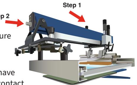
3. Verify that you have the correct off-contact. Your off-contact controls may be towards the base of the press at the center of the carousel. There may be up to four off-contact controls on your screen clamps (two each, left and right). On older presses that do not have built-in off-contact controls, you may need to place a shim made from a wooden paint stick or metal between the bottom of the screen and the bottom of the screen clamp. This will allow for proper screen peel.
