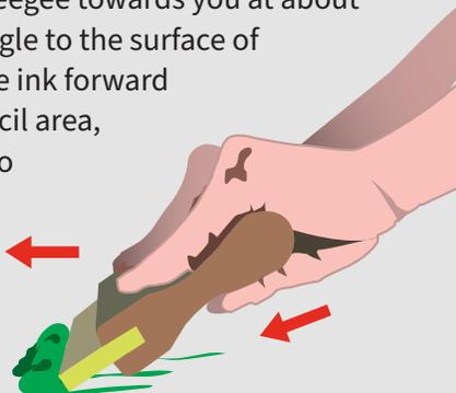
This technique is terrific for holding fine detail on CMYK and simulated process prints and can help control fibrillation.
