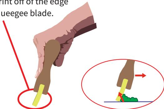
Be sure to flood the screen before committing to your print stroke. Load your screen stencil with the flood stroke and then with adequate pressure, print with the print stroke. The goal is to deposit the ink onto the substrate while simultaneously shearing the top of the ink off.
