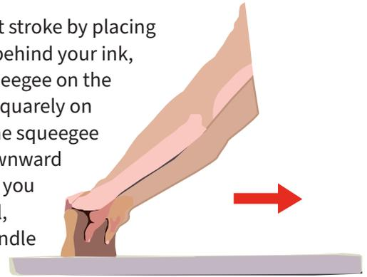
Only the sharp edge of the squeegee should contact the mesh surface. Use enough pressure to clear the ink from the screen, but not so much that you add dot gain and disturb surface fibers.
