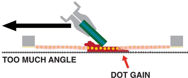
On automatic presses, start with a squeegee angle between 10–15 degrees. On manual presses, begin holding the squeegee behind your ink deposit while resting the blade on the screen surface. From a vertical position resting squarely on the foot of the blade, add downward pressure while beginning to lean the squeegee handle back. Begin your pull, ensuring not to lean the squeegee handle back very far.
