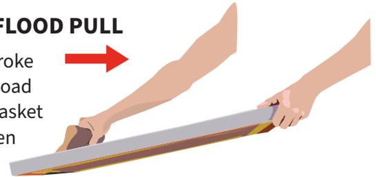
enough ink along the print stroke to lubricate the squeegee blade. This allows the squeegee to move smoothly across the screen mesh.
